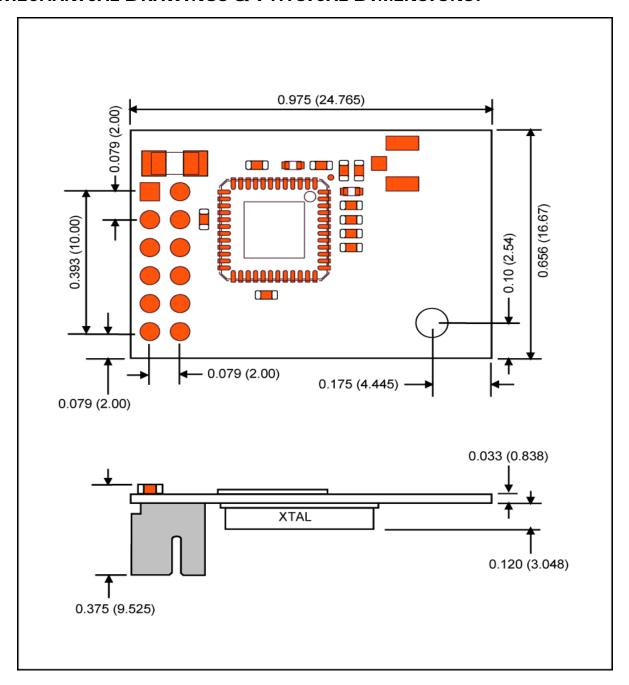
Figure 1 – Juno-M Dimensions (Top View)
